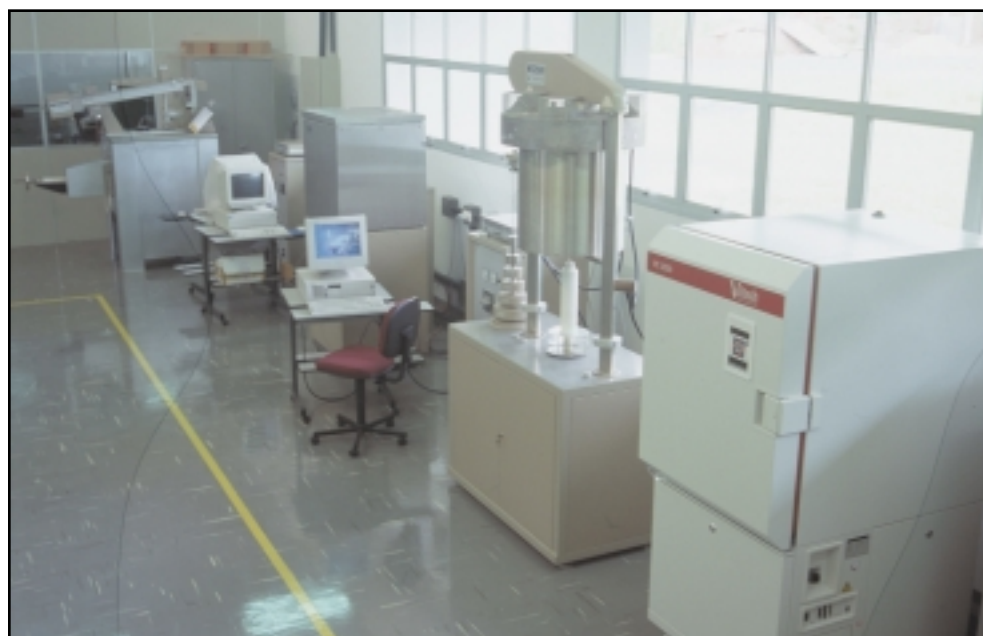
Figure 3. Perspective view of the main DEMa laboratory showing MOR, thermal conductivity and RUL/creep testing equipment.
