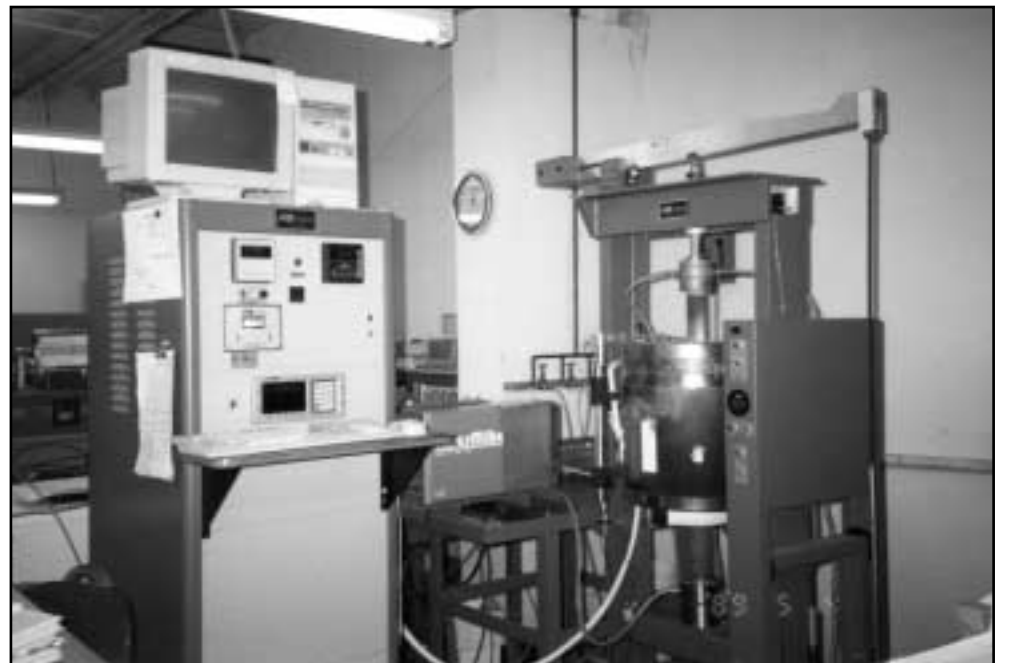
Figure 1 The laser creep testing system at the Orton Refractories Testing and Research Center.
