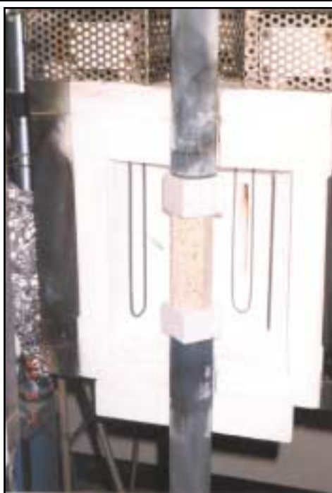
Figure 3 Close-up of the furnace and sample of the laser creep system at Orton Refractories Testing and Center.
