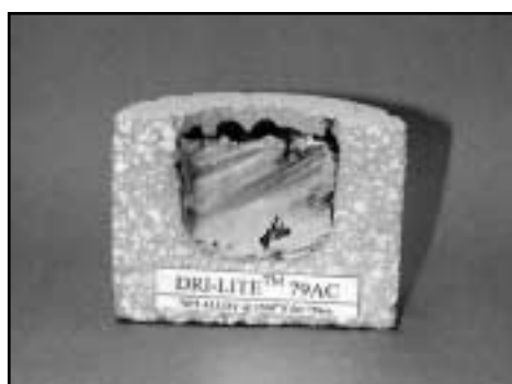
Figure 1. Molten aluminum attack of an insulating dry-vibratable
