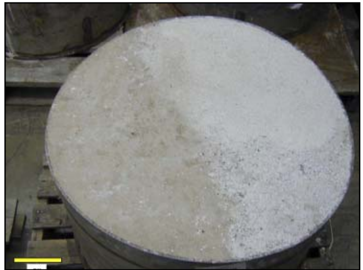
Figure 5. Refractory Coated Manway Plug for Installation at Big Island Commercial-Scale Unit.
