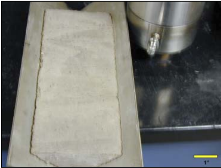
Figure 4. Triangular Prismatic Refractory Sample for Installation in MTCI Fluidized Bed.
