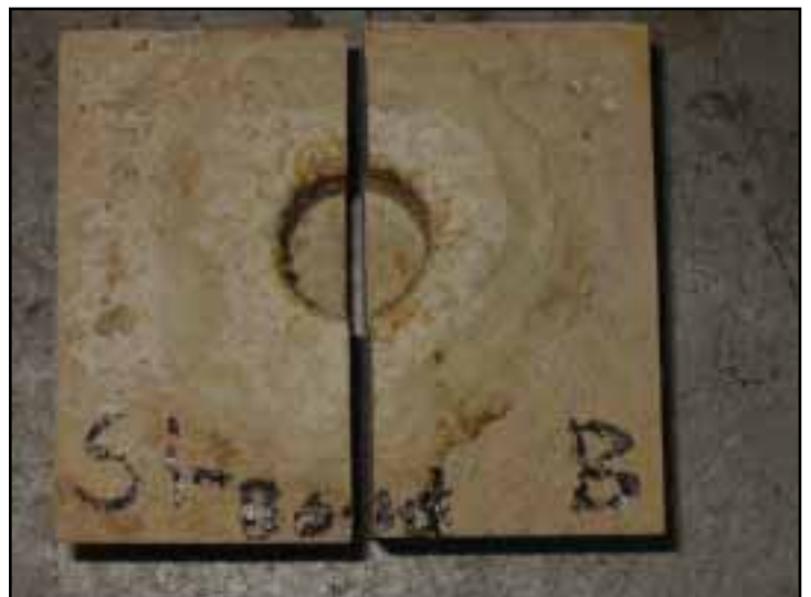
Figure 1. A refractory cup after corrosion test.
