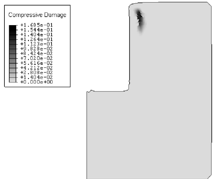
Figure 6. Predicted compressive damage pattern.
