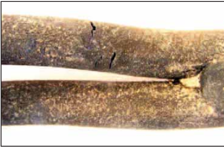
Figure 5. Center anchor cracks near base.
