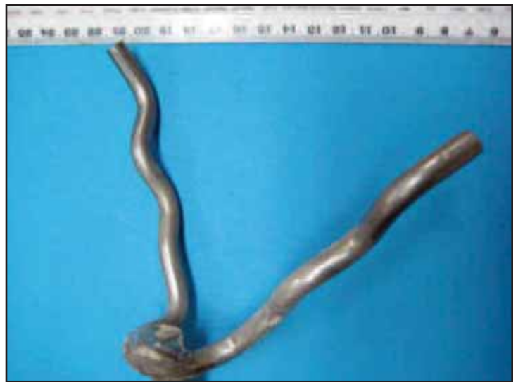
Figure 8. A typical wavy vee anchor.
