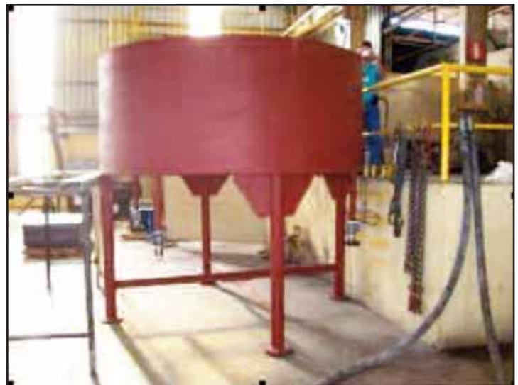
Figure 3. R2U MgO castable installation simulation: Vessel simulating an MPR-L shell.
