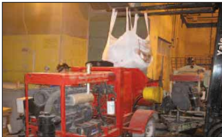
Figure 9. Double piston refractory pumps for installation.
