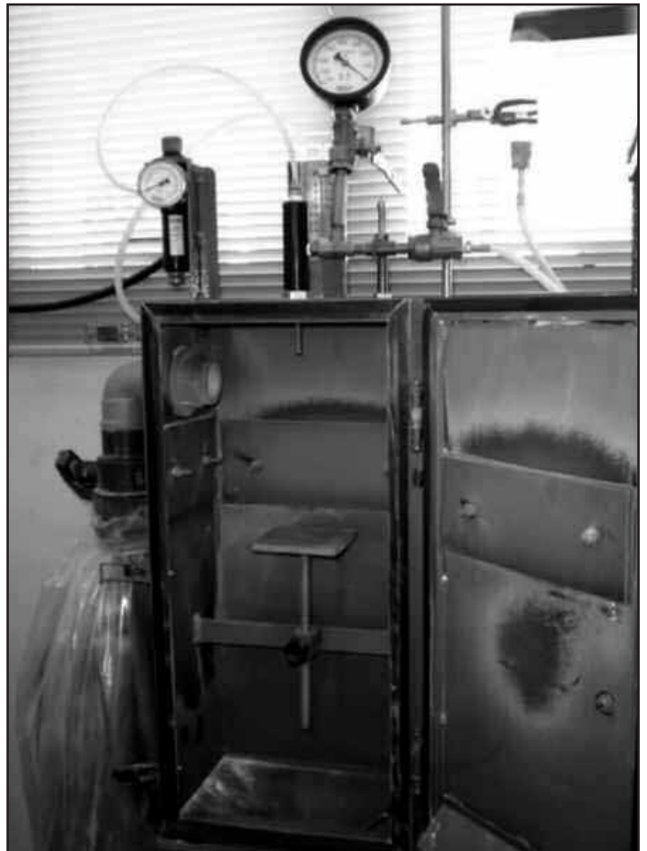
Figure 3. Erosion test equipment [22].
